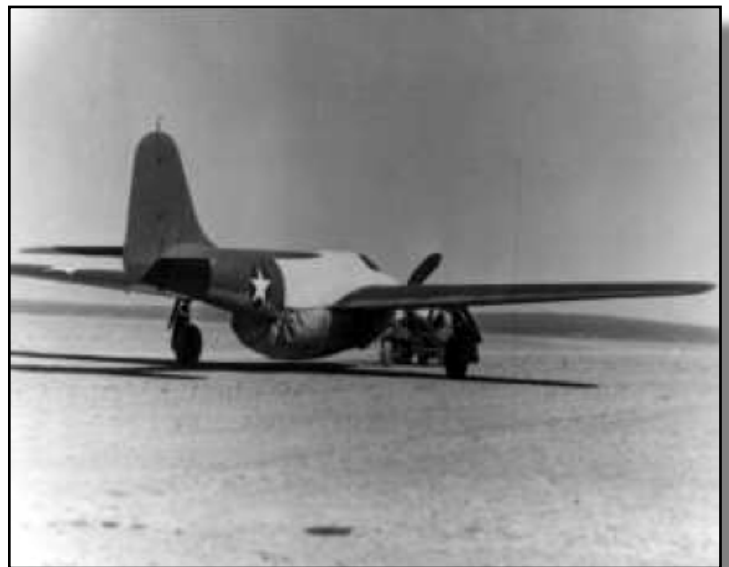
"Bell XP-59A being towed at Muroc Dry Lake, Calif. Note the false wooden propeller designed to conceal the jet engines during ground towing. U.S. Air Force photo"
